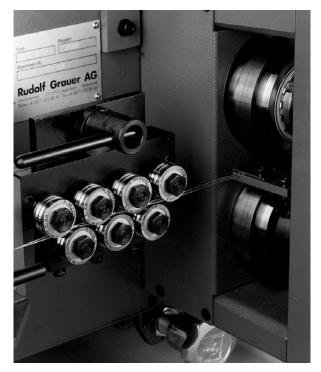
The accurately adjustable feeding system also serves as a flattening unit. The top feed roll can be adjusted on both sides permitting multiwire operation with normal tolerance of wire. The feed length can be set by means of an eccentric and a freewheel clutch. Helical and hardened gears ensure a smooth rolled finish The taper roller bearings on both sides of the feed rolls fully meet the high static and dynamic stress requirements.
