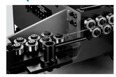
Accurate guidance of each wire is fundamental to a perfect multi-wire process. A straightening system with 7 vertical and horizontal plane rollers, guarantees the necessary straightening quality for the whole range of wire diameters.
